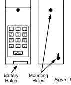
1/8 inch out from the wall. Slide the keypad over the screw and mark the position of the top hole. Remove the keypad and drill the top hole. Slip the keypad back over the exposed screw and finish mounting by installing the top screw. Refer to Figure 1.
