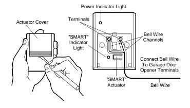
NOTE: If the remote control push button is not held down until the receiver indicator light flashes, the receiver will not learn the code.
