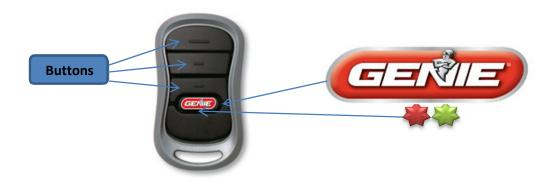
All buttons come factory preset to transmit in dual frequency Intellicode II mode. To confirm that a button is set to this mode, press the desired button. A green LED light above the Genie logo indicates it is in dual frequency 390/315 mode. A red LED indicates it is in 390 Intellicode I mode. **To change modes:** Hold down any button until both LEDs come on (approximately 20 seconds). Release the button and then immediately push it again.
