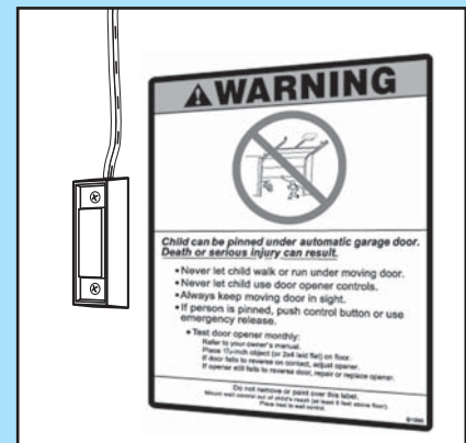
FIG. 3-5 Mounting Entrapment warning label.
