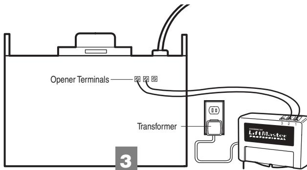
**NOTE:** Transformer Model 85 or 95 is required if your residential garage door opener is a LiftMaster, Chamberlain or Sears.
