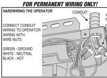
PERMANENT WIRING BETWEEN THE OPERATOR AND THE POWER SOURCE THROUGH A CONDUIT. IT IS RECOMMENDED THAT YOU HAVE A LICENSED ELECTRICAL CONTRACTOR FOLLOW THESE STEPS 1 BE SURE POWER CORD IS UNPLUGGED.
