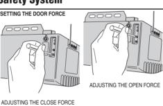
USE A SCREWDRIVER TO ADJUST THE LIMIT
