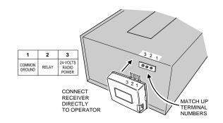
STEP 1B MDRG Installation (For non 24V Operator). A Model TF524 step-down transformer must be used to power the receiver when connecting to an operator supplying anything other than 24V. Install the screws supplied into the brass terminals on the receiver. Connect the transformer wires to Terminals 1 & 3 (polarity not important). Connect receiver Terminals 1 & 2 to the two operator activation terminals (polarity not important).
