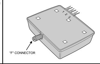
STEP 4 MDRG Program button and LED Location. Locate the program button and LED on the side of the receiver case.
