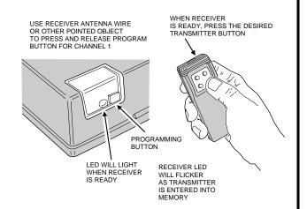
**STEP 6** Add additional transmitters. Repeat Step 5 for each transmitter used with this receiver. Be sure to press the receiver's program button *each time* a new transmitter or a different transmitter button on a multi-button transmitter is pressed. If the LED doesn't come on when the receiver's program button is pressed, the receiver's memory is full (40 transmitters total). Use the erase function (Info 1) to remove transmitters from the receiver's memory.
