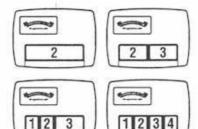
Set switches 1 through 9 at any security code, press and hold desired channel. Now press learn. The green LED will flash indicating the channel is stored. One flash is for channel one, two for channel two, three for channel three, and four for channel four. The transmitter has now stored the code in the corresponding channel until the learn switch is pressed again.
