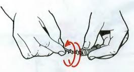
Make sure cable will not pull out of spring.
