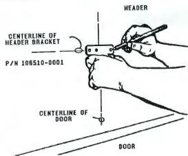
Drill 5/32" diameter holes at marked locations.
