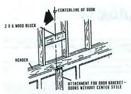
If header does not have suitable woodwork where header bracket will be installed, then such will have to be made. It is suggested that a wood 2"x6" be secured to nearby woodwork.
