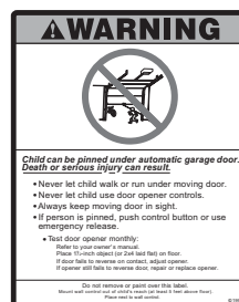
Entrapment Warning Label
