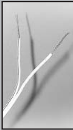
FIG. 3-6 Splitting and stripping.
