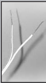
FIG. 3-6 Splitting and stripping.
