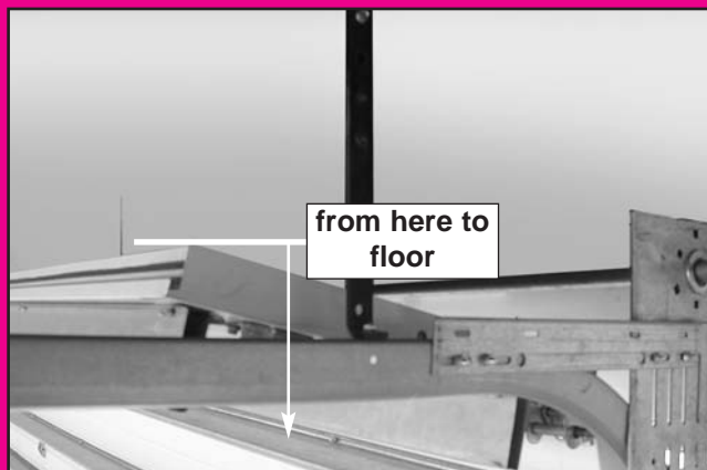
FIG. 2-1 Finding highest point of travel (sectional).
