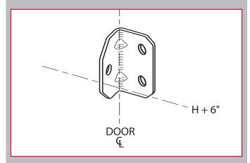
Fig. 1-24 Header bracket orientation
