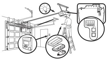
Press and release the "learn" button on the motor unit. The learn indicator light will glow steadily for 30 seconds.
