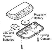
Replace the batteries with only 3V2016 or 3V2450 coin cell batteries.
