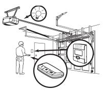
Press the PROG <Learn> button on the Smart Control Panel<sup>™</sup>.
