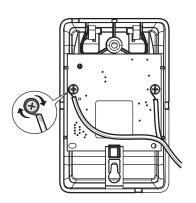
**PRE-WIRED INSTALLATIONS:** Choose any two wires to connect, but make note of which wires are used.
