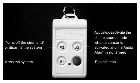
When the Audio Alarm is ON, the four buttons on the transmitter do the following:
